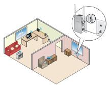
Set the Access Point/Extender switch to Access Point ........ 1.
