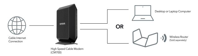
Connect the CM700 High-speed cable modem directly to your computer, or your WiFi router for connecting to wireless devices.
