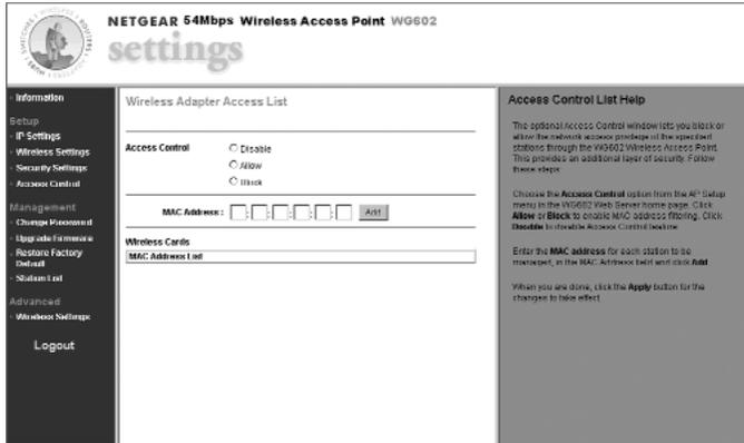
The optional Access Control window lets you block or allow the network access privilege of the specified stations through the WG602 Wireless Access Point. This provides an additional layer of security. Follow these steps:
