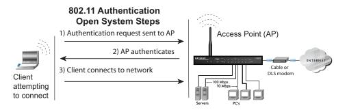
Figure 4-1: 802.11 open system authentication
