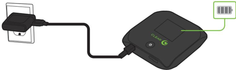
4. After your Clear Spot is completely charged, turn on the Clear Spot by pressing and holding the Power button for 2-3 seconds. The device will automatically activate when a 4G network is acquired. When activation is successful, the LCD will briefly display "Activation complete" before trying to establish a network connection.
