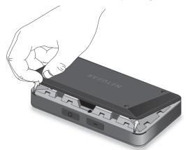
2. Insert the battery as shown, ensuring that the gold contacts on the battery line up with the gold contacts on the hotspot.
