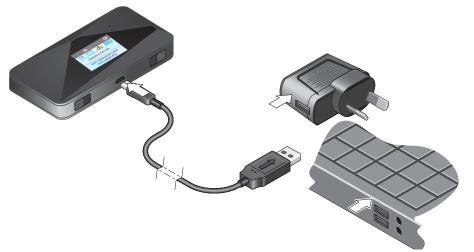
2. Plug the wall charger into a wall socket.
