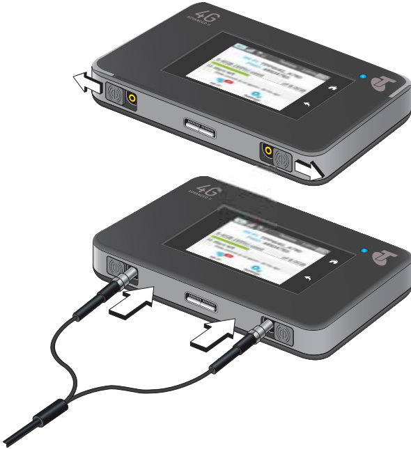
Figure 4. External antennas with TS-9 connectors
