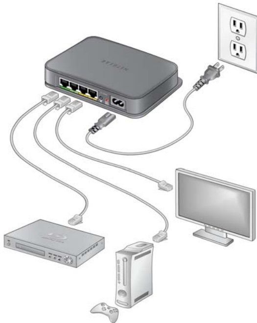
Figure 4. Connecting devices to an XAV5004 Powerline adapter
