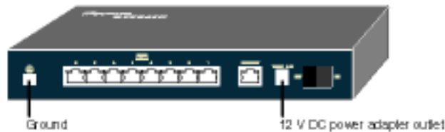
Figure 2-2. RO318 Rear Panel
