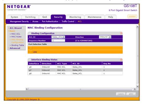
You can assign an optional sequence number to indicate the order of this access list relative to other access lists if any are already assigned to this interface and direction.
