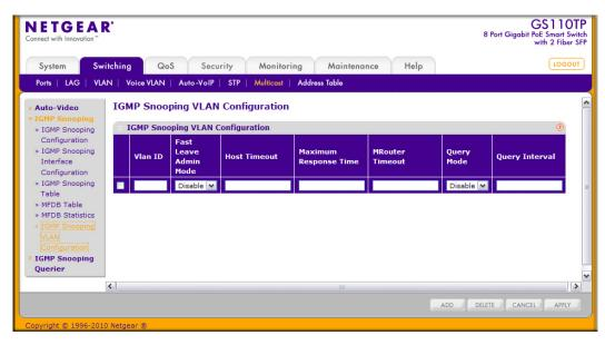
To configure IGMP snooping settings for VLANs:
