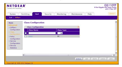
The class name is a hyperlink. The following figure shows the configuration fields for the class.
