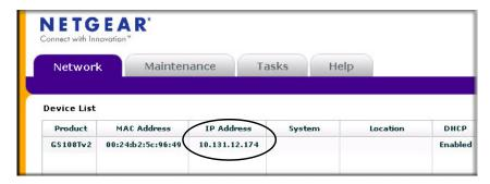
7. Select your switch by clicking the line that displays the switch, then click the Web Browser Access button. The Smart Control Center displays a login window similar to the following figure.
