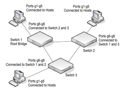
Perform the following procedures on each switch to configure MSTP:
