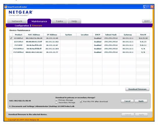
By default, the firmware is downloaded to primary storage and will be become the active image after the download completes and the switch reboots. To download firmware to use as a backup image, select the **Secondary Storage** option. To prevent the switch from using the downloaded firmware as the active image, make sure the Run this FW after download option is clear.
