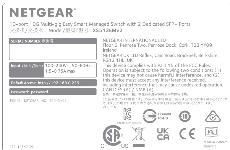
Figure 4. Switch label model XS512EMv2
