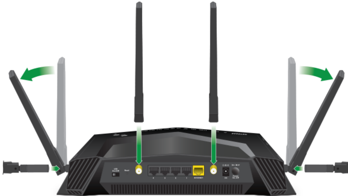
Figure 4. Attach the antennas and position them for best WiFi performance
