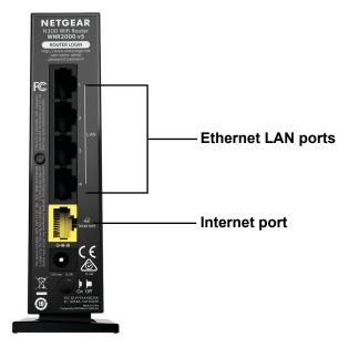
Do not connect this Ethernet cable to the yellow Internet port on the router.
