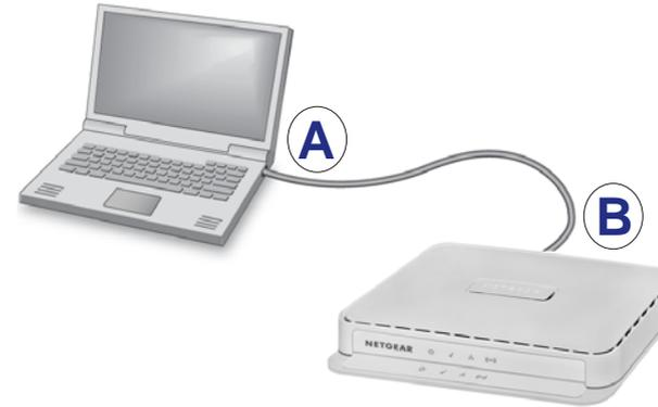
2. Insert an Ethernet cable in the Ethernet port of the computer (point A in the illustration).
