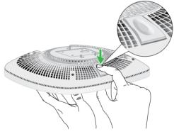
3. Turn the AP counterclockwise until the AP releases from the mounting plate. The mounting plate remains attached to the T-bar or the wall.
