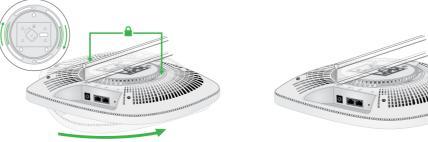
8. Twist the access point clockwise to lock it onto the mounting plate.
