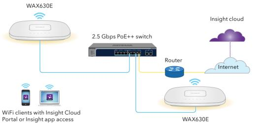
Sample connections for a standalone setup
