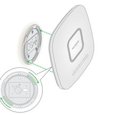
8. Twist the AP clockwise to lock it onto the mounting plate.
