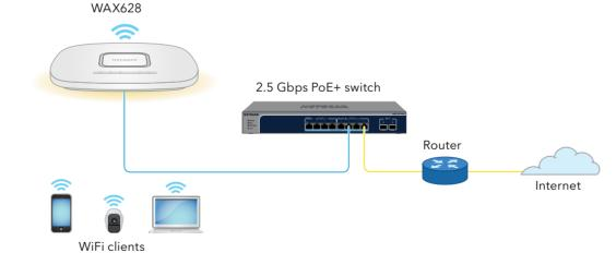
If connected to 2.5 Gbps equipment, the WAX628 LAN 1/PoE+ port supports Ethernet speeds up to 2.5 Gbps within your LAN. The preceding figures show a NETGEAR MS510TXUP switch, which supports speeds of 2.5 Gbps and higher, as well as PoE+. If your Internet connection, modem, router, and switch support a speed of 2.5 Gbps, the AP's Internet connection also functions at 2.5 Gbps. Otherwise, the Internet connection functions at 1 Gbps, which is a common speed.
