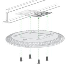
7. Hold the AP upside down and attach it to the mounting plate.
