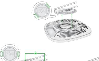
8. Twist the AP clockwise to lock it onto the mounting plate.
