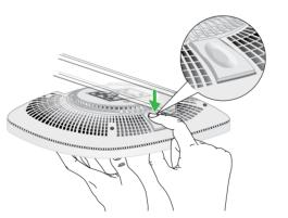
3. Turn the AP counterclockwise until the AP releases from the mounting plate. The mounting plate remains attached to the T-bar or the wall.
