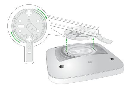
8. Twist the AP clockwise to lock it onto the mounting plate.
