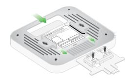
3. Slide the AP into the bracket until it locks in place. The locking tab must be at the front of the AP.
