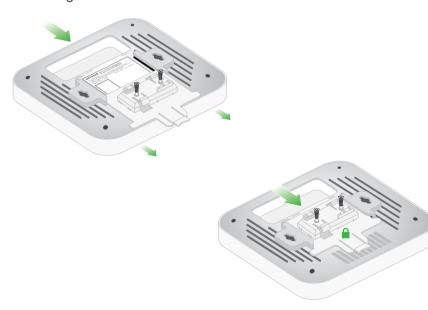
Note: To unlock the AP, push the locking tab toward the ceiling and slide the AP out of the bracket.
