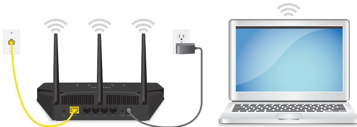
Figure 6. Connect the AP to an Ethernet wall outlet with Internet service
