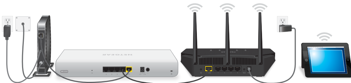
Figure 5. Connect the AP to an existing router in your network
