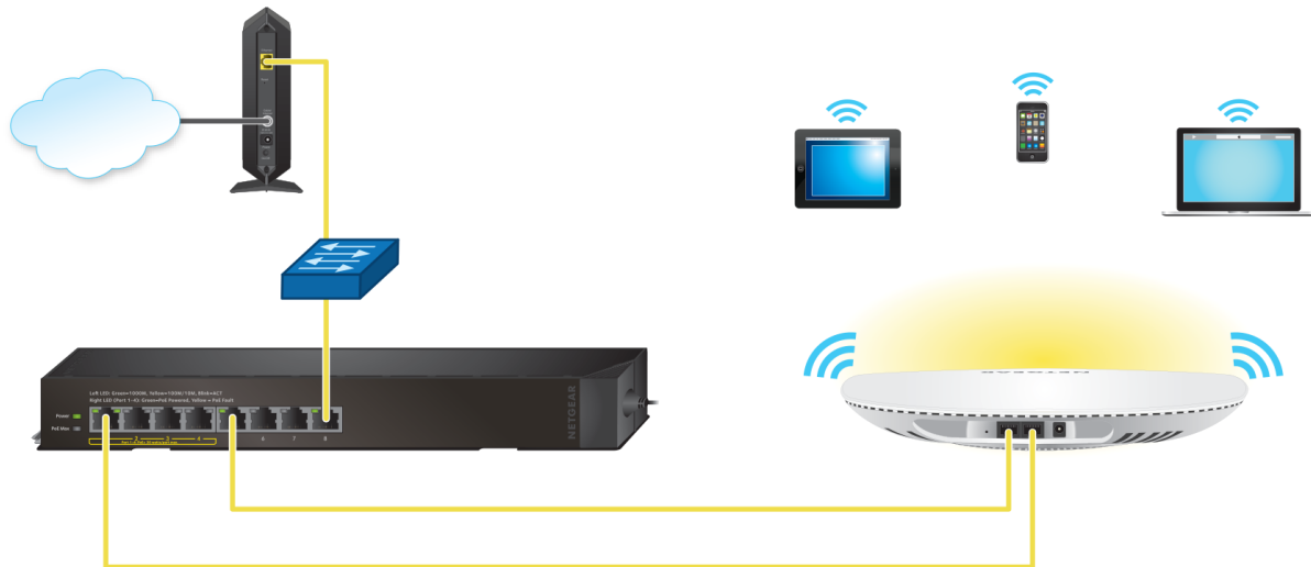
Figure 9. Link aggregation connection
