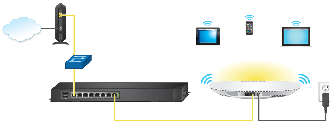
Figure 5. Set up the access point with a connection to your network
