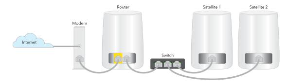
Figure 5. Ethernet backhaul connection using a switch
