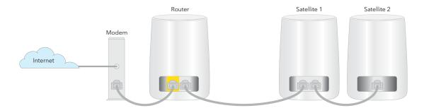
Figure 4. Daisy chain topology: Satellite 1 connected to router and satellite 2 connected to satellite 1
