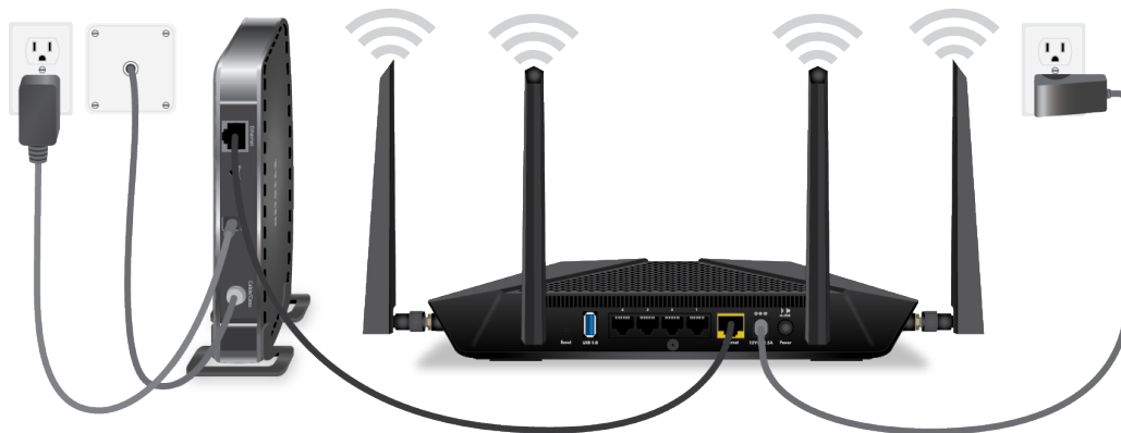
Figure 7. Cable your router
