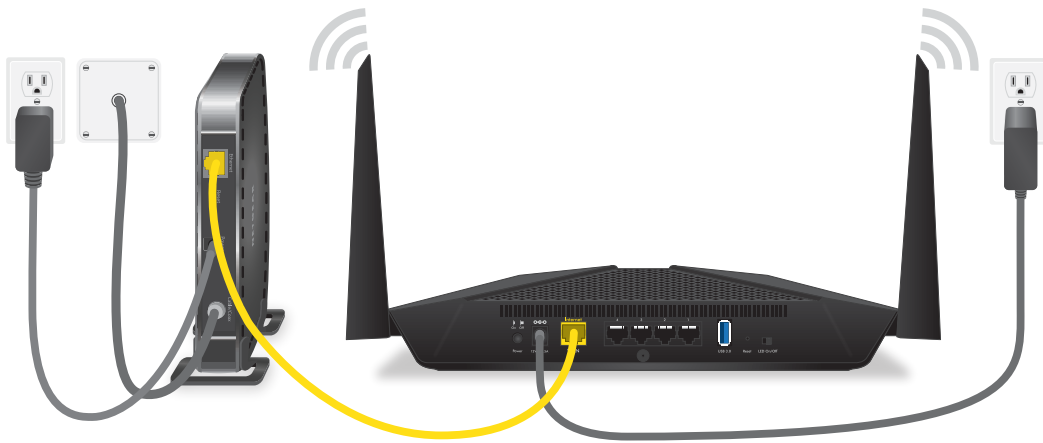
Figure 5. Cable your router
