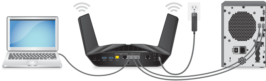
Figure 7. Ethernet port aggregation to a LAN device
