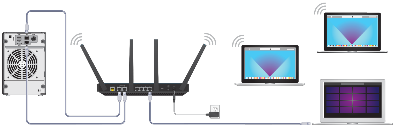
Figure 11. Ethernet port aggregation
