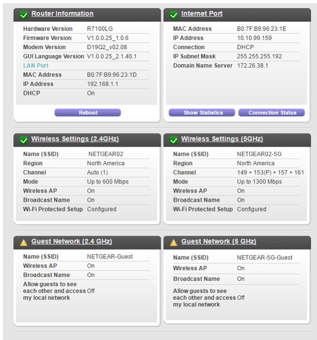
Your modem router might display information that is different from this example. If your router is set up to lease an intranet address from your Internet service provider (ISP), the Internet Port pane displays the IP Address, Connection, and Subnet Mask intranet values in parentheses.
