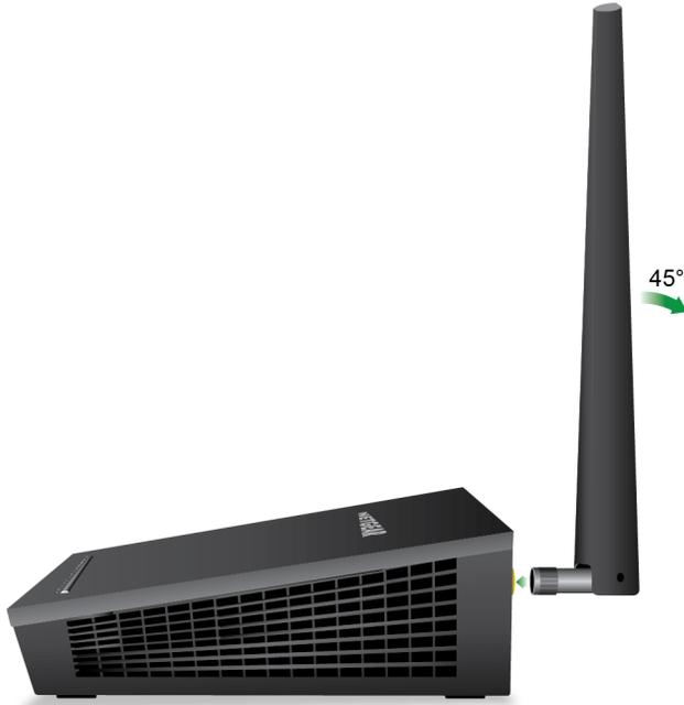
2. Attach the antennas on the threaded antenna posts.
