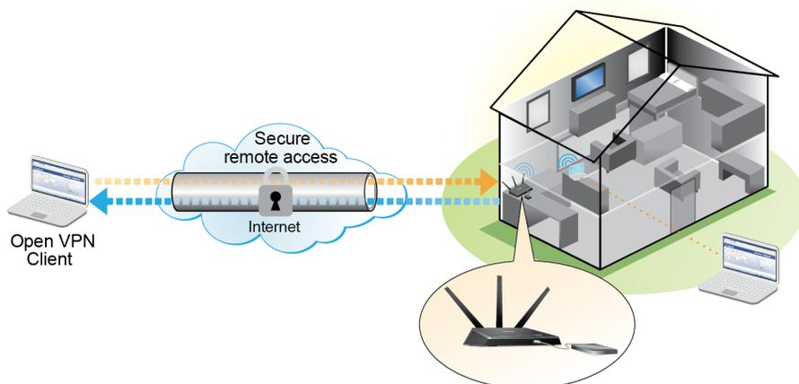
This type of VPN access is called a client-to-gateway tunnel. The computer is the client, and the router is the gateway. To use the VPN feature, you must log in to the modem router and enable VPN, and you must install and run VPN client software on the computer.
