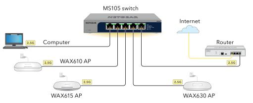
NOTE: Each connected device requires a power adapter because the MS105 switch does not provide PoE power.
