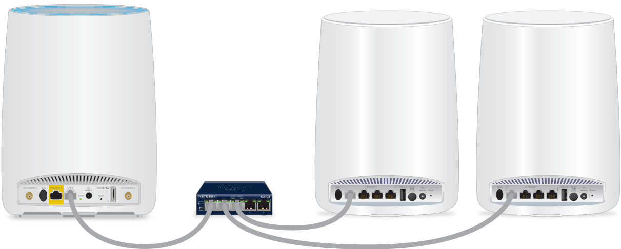
Figure 4. Ethernet backhaul connection using a switch
