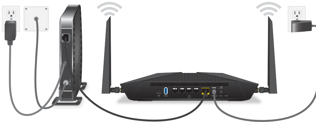
Figure 7. Cable your router
