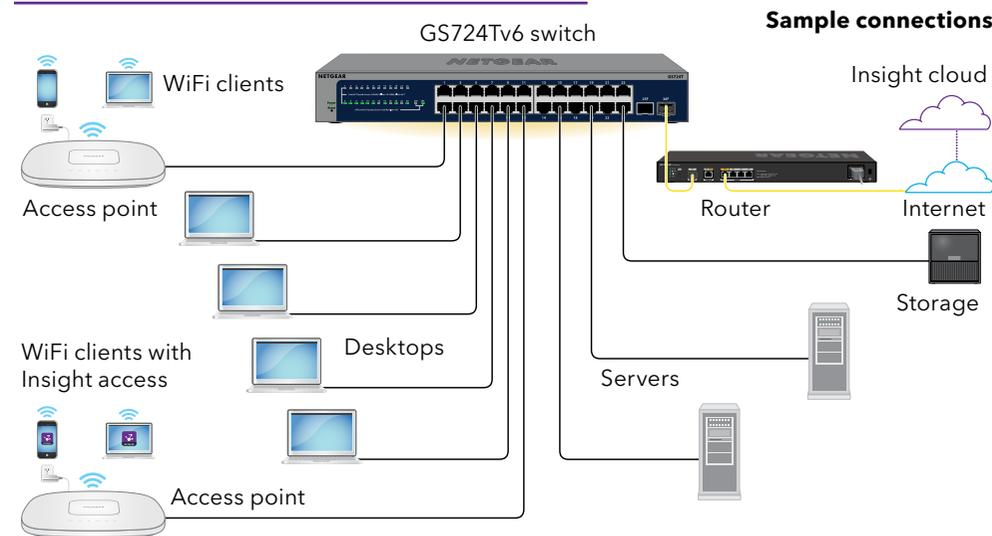
1. Connect devices to the RJ-45 Gigabit ports on the switch front panel. Use Category 5e (Cat 5e) or higher rated Ethernet cables terminated with RJ-45 connectors to make connections.
