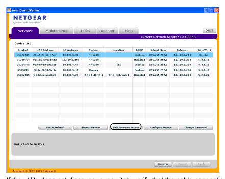
If the utility does not discover your switch, verify that the cable connections are secure and that the IP address configuration of the computer is in the same subnet as the switch, and click the **Discover** button.
