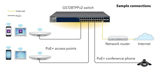
This switch is designed for indoor use only. If you want to connect to a device located outdoors, the outdoor device must be properly grounded and surge protected, and you must install an Ethernet surge protector inline between the switch and the outdoor device. Failure to do so can damage the switch.
