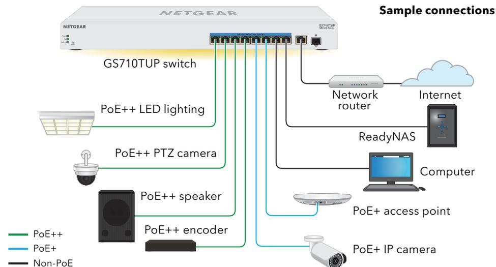
This switch is designed for indoor use only. If you want to connect to a device located outdoors, the outdoor device must be properly grounded and surge protected, and you must install an Ethernet surge protector inline between the switch and the outdoor device. Failure to do so can damage the switch.
