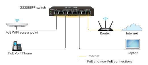
Note: We recommend that you use a Category 5e (Cat 5e) cable or higher-rated cable for Gigabit Ethernet connections.
