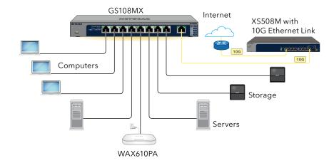
**NOTE:** We recommend that you use a Category 6a (Cat 6a) cable or higher-rated cable for 10-Gigabit Ethernet connections, and a Category 5e (Cat 5e) cable or higher-rated cable for other Gigabit Ethernet connections.
