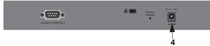
3. Connect the power adapter to an electrical outlet. The Test LED (5) lights and turns off.
