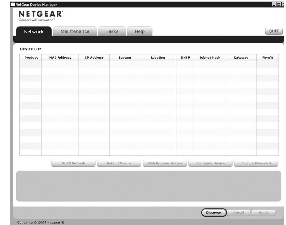
2. Click the **Discover** button. The Smart Control Center Utility finds the switch and displays its MAC address, IP address, and model number. If the utility does not discover your switch, verify that the cable connections are secure and that the IP address configuration of the computer is in the same subnet as the switch, and click the **Discover** button.
