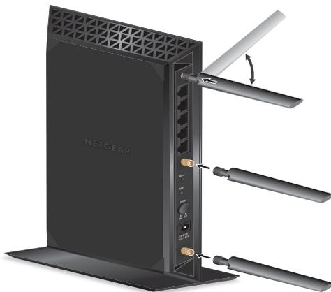
2. Attach the antennas on the threaded antenna posts.
