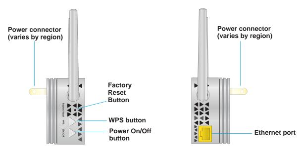
Figure 2. Buttons and port on the side panels
