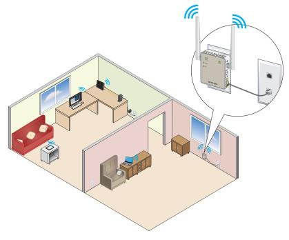
Figure 5. Extender in access point mode
