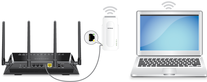
Figure 4. Extender in access point mode
