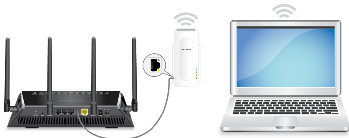
Figure 4. Extender in access point mode
