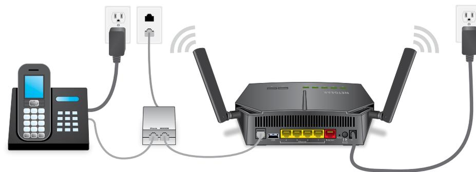
Connect the DSL port on the modem router to a DSL outlet.
