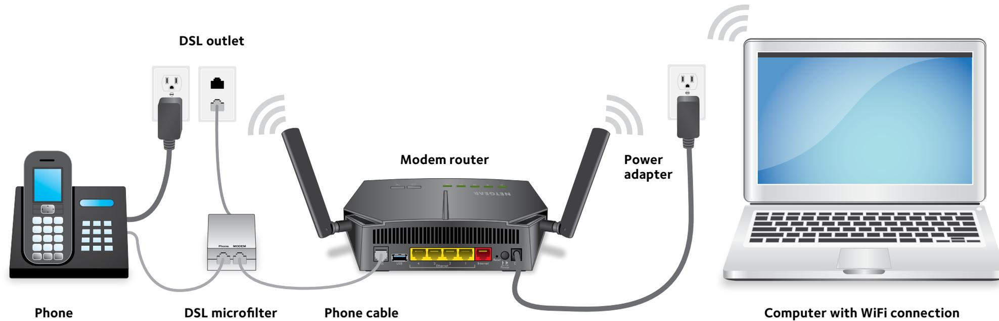
**Note:** To connect to the modem router, you can use either a computer with an Ethernet cable connection or a computer with a WiFi connection.
