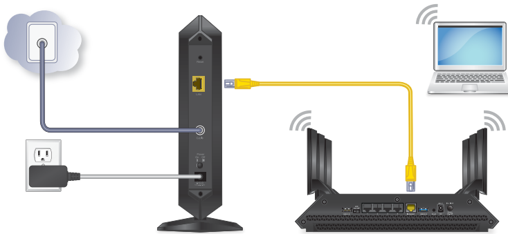
Figure 7. Connect the cable modem to a router
