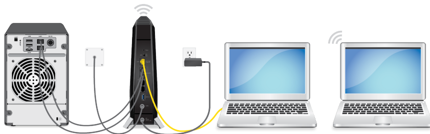
Figure 4. Ethernet port aggregation
