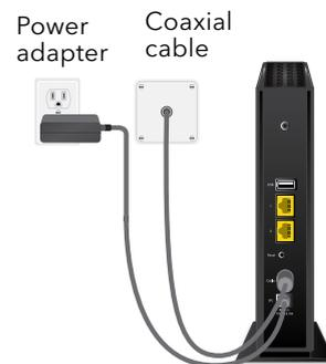
We recommend connecting directly to the cable wall outlet. If you must share the connection, use a 3.5dB (1 to 2) splitter.
