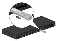
2. Lift the latch on the module to lock it in place.
