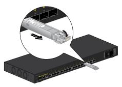
2. Grasp the sides of the module and pull it straight forward out of the slot.
