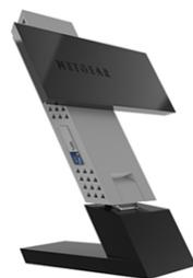
In this position, the internal antennas are extended out from the adapter for increased WiFi performance.
