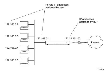
Figure 10-3. Single IP Address Operation Using NAT
