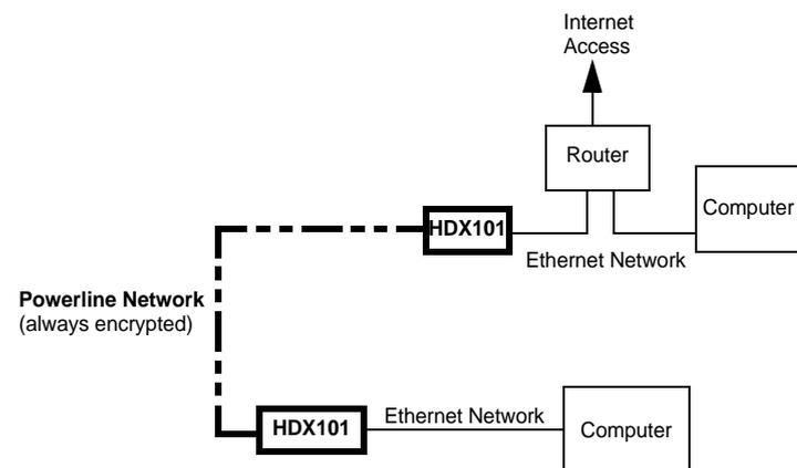
The encryption of the information you send over the Powerline helps keep it secure. This security feature is especially relevant in settings like apartment buildings.
