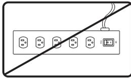
Do not connect the HDX101 to a power strip, extension cord, or surge protector as this may prevent them from working properly or degrade the network performance.
