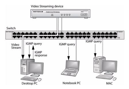
Figure 22-1 IGMP Querier Directing Video Stream
